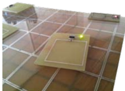
Multiple devices powered wirelessly from a metamaterials platform
