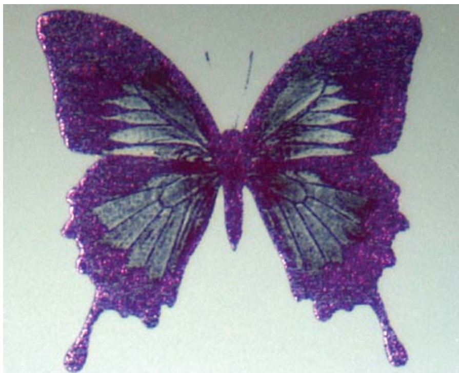
Example of an electrically constructed image, 70 \mu m wide, on a phase change material optoelectronic film
