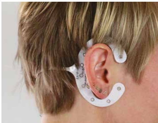
Figure 1: The cEEGrid array. For better signal quality, an array can be placed around each ear. The cEEGrids interphase over bluetooth with a smart phone, that stores the recording.
