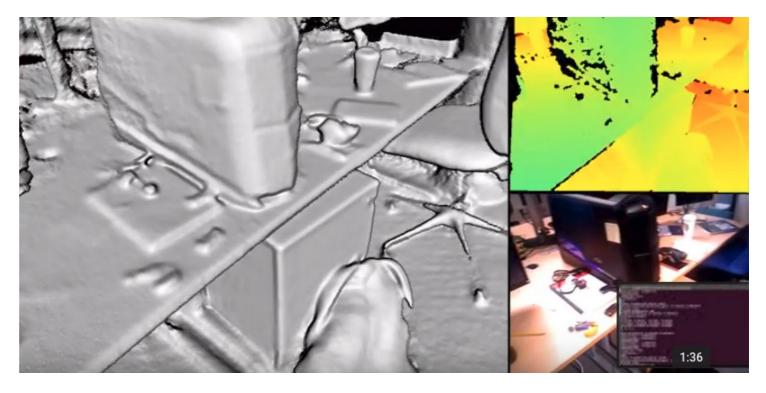
Researchers at Oxford have developed an algorithm that uses a single RGB-D frame as an input to estimate the respective 6-D camera pose relative to a map built beforehand, which can be used with a SLAM or VR/AR system.
